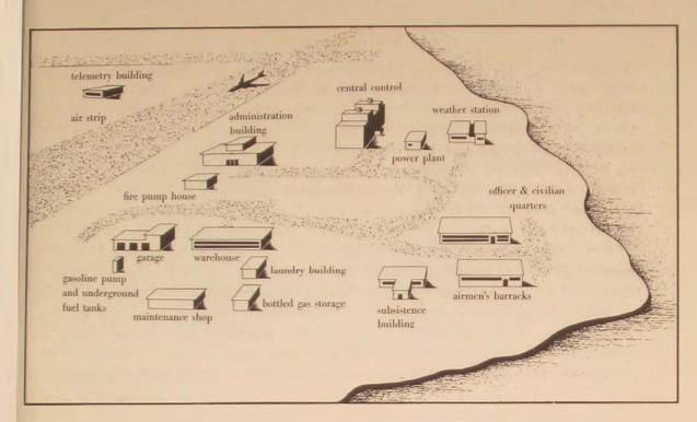
The typical down-range station consists of the elements shown in this diagram. Aside from the essentials of auxiliary air base support, the bulk of the equipment is electronic—both radio and wire communications, the surveillance radar, the guiding and tracking radar, and the electrically-controlled optical tracking equipment. The landing strip provides for communication with the other islands and the mainland and is used by the "Polly" aircraft that assist in general range clearance.
