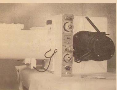
The CZR-1 Bowen camera, like the Clark Ribbon Frame camera, is set up at the launching site to take micro-second photographs of the vehicle during the first twoand-one-half seconds of flight.
